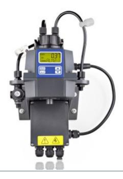
Turbidity measurements with DULCOTEST DULCO turb C: Compact measuring instrument that uses light scatter to measure turbidity, with a large measuring range and different designs to comply with ISO and EPA standards. Available with or without automatic cleaning.
